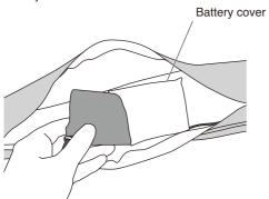
③Cut all the cords extending from the rechargeable battery using scissors. Never remove the insulation film from the removed battery; doing so may cause an electric shock or short.
