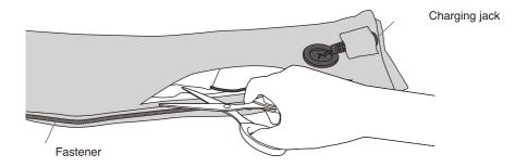
②Remove the rechargeable battery from the battery cover.
